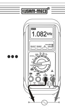
Function defaults at VFD-ACV\*\*\*. By default, voltage is set at 600V & 1000V two auto-ranges to best cope with most Variable Frequency Drives (VFD) measurements. High noise-rejection frequency measurement algorithm and Low-pass filter circuit are permanently bundled with all voltage and frequency function-ranges within this rotary-switch position. Press the RANGE button momentarily to select other ranges only when needed.
